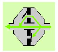
Many contemporary Citroëns—including both regular hydropneumatic and Hydractive Xantia and XMs—have an anti-sink system (SC/MAC) fitted, to keep the car from lowering when not used. The system does not interfere with the normal functioning while in use. It attempts to minimize leaks inside the system by having only one element that can leak, the anti-sink valve itself.
